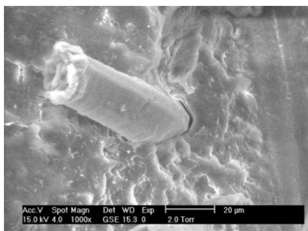
Figure 10 Fracture surface of flax fiber-reinforced PP-EPDM composites.
